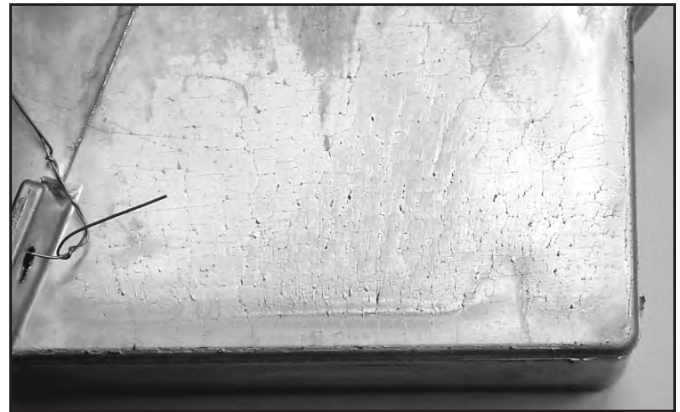
Figure 2-14 Washout as seen on a casting.
