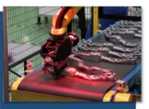
The addition of the robot allows the operator to shift focus to other tasks, including cosmetic inspection, gauging, or tending other machines. Several hours' worth of machined product can be loaded/unloaded in seconds onto the side-by-side input/output conveyors that are integrated into the cell and tied into the robot's logic.
