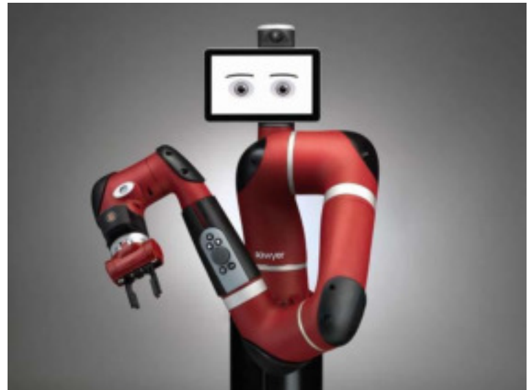
Rethink Robotics’ Sawyer Sawyer™, a smart, collaborative robot scheduled for limited release this summer, is designed to execute precise tasks—such as machine tending and circuit board testing—that have, historically, been impractical to automate with traditional industrial robots. (PRNewsFoto/Rethink Robotics)
