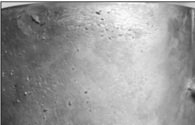
Figure 2-11 Heat checking as seen on a casting.
