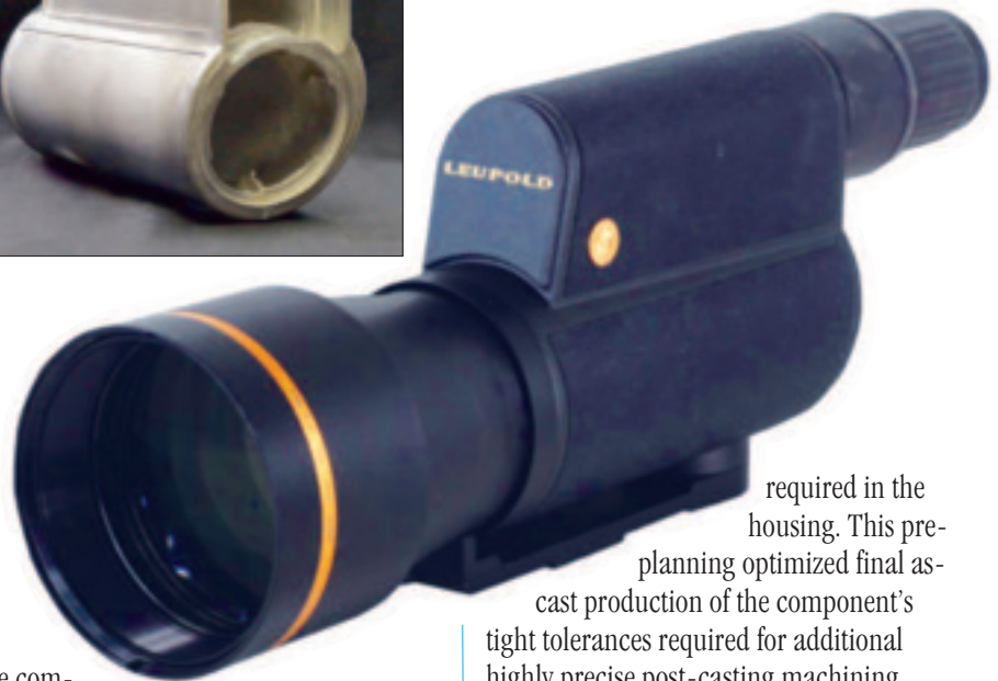
Compact spotting scope's central housing (left), die cast in AZ91D magnesium alloy, weighs 8 oz. with selected wall sections to 0.039 in., as-cast. Completed scope assembly shown below.
