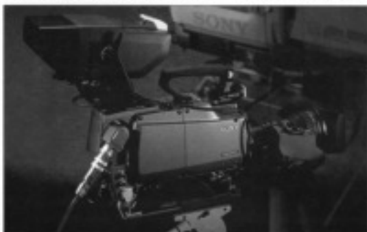
This Sony professional video camera for field telecasting was designed with Al and Mg die castings to meet the requirements for high strength, compactness, low weight, rigidity, EMI/RFI shielding, and a cosmetic surface finish on the enclosure exterior. The 11 CWM cast parts, shown at upper right, will be featured in CWM color ads in leading OEM product design publications.
