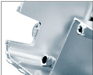
Gripper projections of 0.200 x 0.050 x 0.040 in. "lock" the overmold to the die casting.
