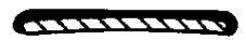
Improved Design. Use 0.015 in./in. crown to hide undulations caused by uneven buffing.
