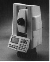
Using pulsed laser electronic distancing technology, the new Trimble TTS 500 optical surveying instrument (above) incorporates four Mg die cast components (left) to achieve stiffness and ruggedness, with light weight. Mg provides the highest strength-to-weight ratio of any commonly-used engineering material.
