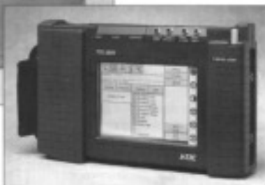
The portable T-BERD 2209 Communications Analyzer, above, is designed with a die cast display frame, left, to take the shocks of rugged field use. Mg die casting was the choice over all other materials and processes.
