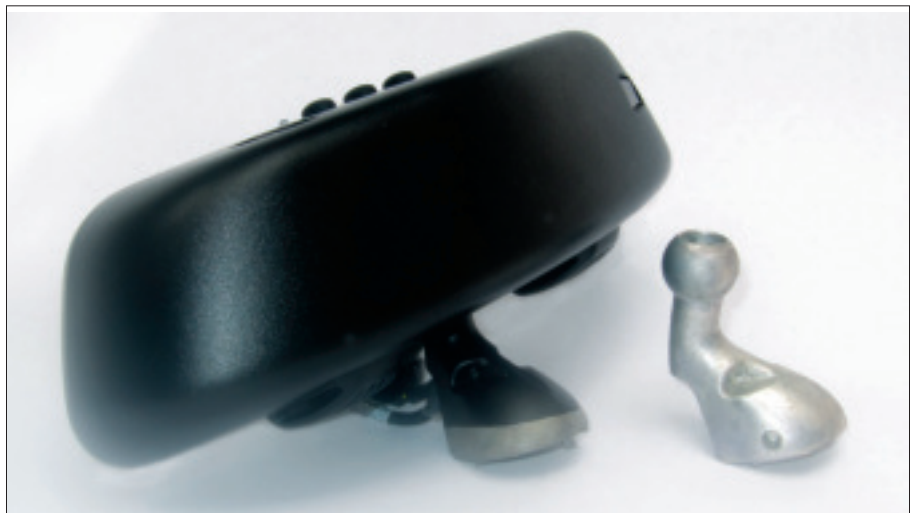
Mirror-mount support (right) requires critical dimensional accuracy and structural integrity for operation over wide ranges of temperature and humidity. Ball-end tolerance is held to \pm 0.1 mm.
