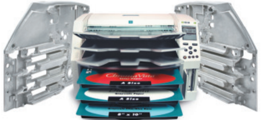
Imager's Mg die cast side walls are 12 x 17 in. CWM CNC precision machining brings positioning tolerances of \pm 0.001 in. for select locations and flatness to 0.025 in. across a zone of 9 x 14 in.
