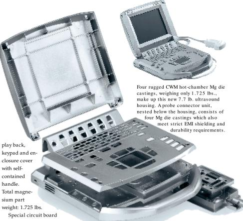
Special circuit board design, tight-fitting die cast housing joints and magnesium's built-in shielding characteristics provide total EMI/RFI isolation without the use of additional plating or EMI gasketing.
