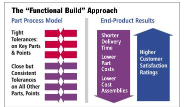
Conventional manufacturing calls for each part to strictly pass the socalled Cpk. In "Functional Build," parts tight on key points, close on all others, are used, with overall assemblies held to tighter tolerances.
