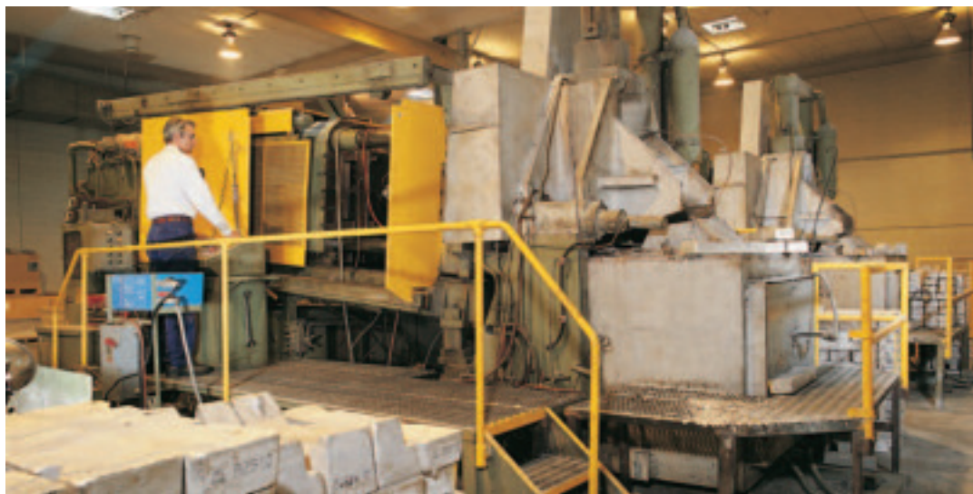
Two of our largest hot-chamber magnesium die casting machines, 650-ton Frechs, can cast 24 in. x 24 in. (60.9 x 60.9 cm) Mg parts using the more cost-efficient hot-chamber process—resulting in closer-toleranced, corrosion-resistant castings at the weight of molded plastic.
