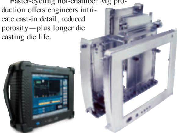
Magnesium and elastomer overmold for a fiber optic cable tester is the first known soft-touch overmolding of a complex die cast case. It provided assured EMI shielding and a shock-resistant exterior with high impact strength—superior to plastic at a 20% saving.
