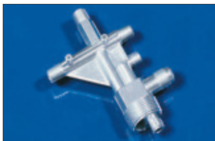
Zinc die cast air compressor valve was produced with seven external thread sets cast in place. The high-tech die casting resulted in an 85% unit cost reduction over the six-part aluminum and brass assembly it replaced. Tooling payback was less than 6 months.
