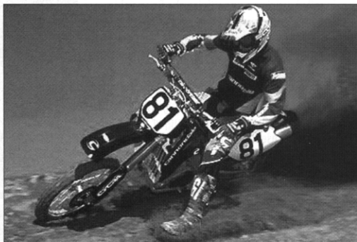
Breaking traditional motocross design rules, the new MX400 boasts an innovative reversed-position four-stroke engine. A version of the 432cc four-stroker is also being used to power a new line of FX400 quad ATVs.
